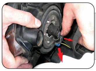
Open hood. Look down from above into the engine bay and locate the low beam bulb. Remove retaining clip on the low beam by simultaneously unclipping and pulling the connector away from the bulb.
