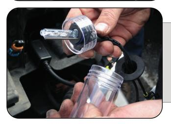
Remove the HID bulb from the protective plastic casing and screw cap. Do not touch the bulb with your bare hands. If you do, be sure to clean the bulb with rubbing alcohol prior to installation.
