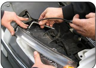
Reinstall headlight assembly if removal was required.
