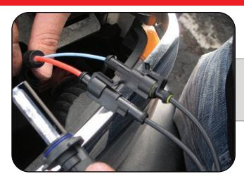
Connect corresponding AMP connectors from the ballast to bulb.
