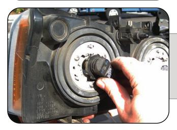
Twist OEM bulb counter clockwise to unlock the bulb from headlight housing. Once the bulb is unlocked remove gently from housing.
