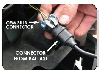
Insert the male connector (the connector that came out of your OEM bulb) into the female connector coming out of the ballast. Mount ballast with the double sided tape provided to a clean flat surface in the engine bay.
