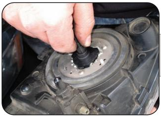
Twist bulb clockwise into place locking it securely into the headlight housing.
