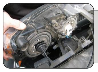
Slide the rubber grommet up to the bulb plug which keeps the bulb protected from the elements.
