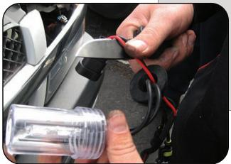
Adapter harnesses are not necessary for this HID installation. If desired you can cut and remove the adapter harnesses as pictured to left.
